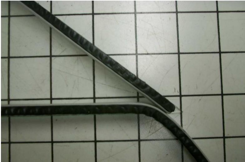
Figure 7: Start application at the sharpest corner of an odd-shaped unit.
