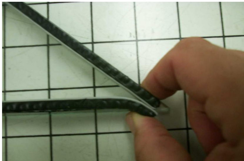
Figure 8: Pinch the corner to seal the unit
