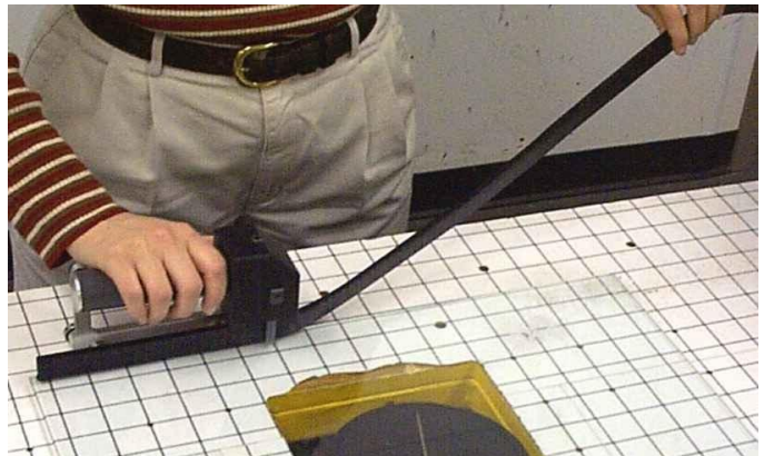
Figure 11: Hold the spacer lightly, and slightly above and off the glass edge.
